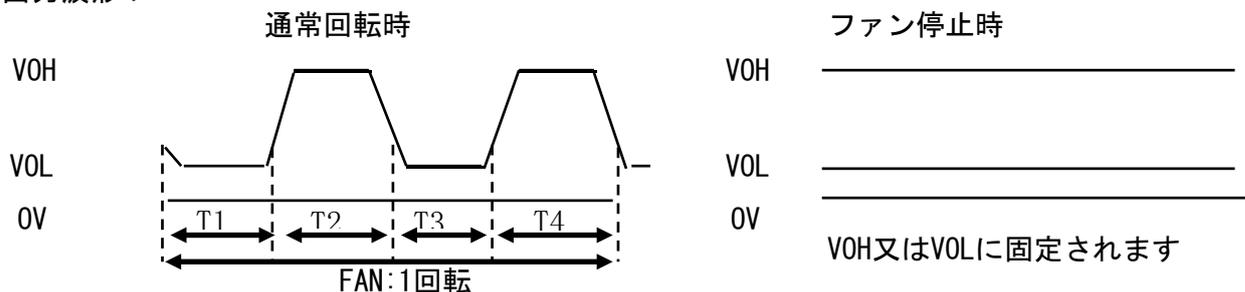
$T1 \sim T4 = 60/N [\text{sec}]$      $N = \text{FAN回転速度} [\text{min}^{-1}]$
